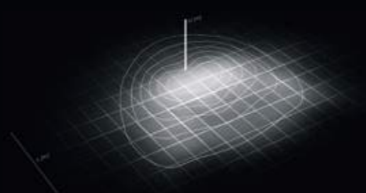
LT-64 Asymmetric Beam with backlight L / H = 2
